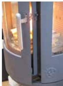
4. When you can see that the chimney is hot enough to draw (after 5 - 10 minutes), close the door. If all the necessary conditions are met, a thick layer of embers will have been formed in the combustion chamber after another 15 - 20 minutes, and there will be a high temperature in the combustion chamber, which is necessary in order to be able to continue the combustion.
