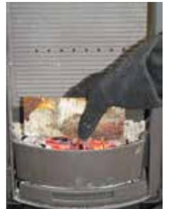
The stove door must be opened gently the first 2 - 3 centimetres, then you should wait until the pressure has equalised before opening the door all the way. This technique will prevent smoke from getting out, particularly when there is a poor draught.
